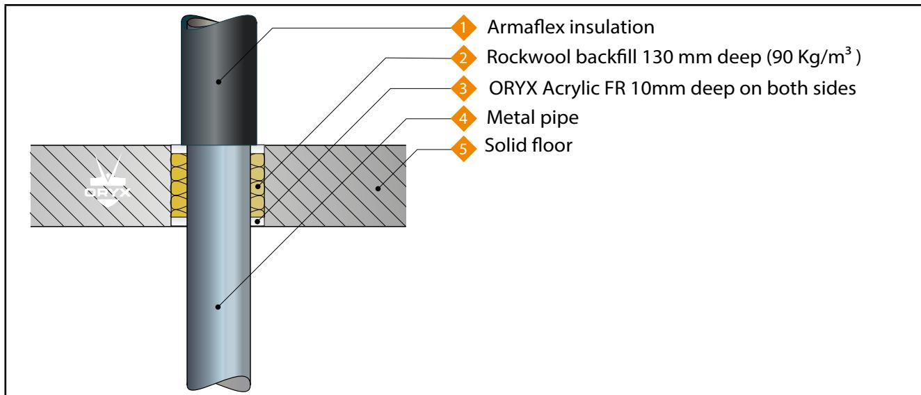
**A.1.1.1 Pipes with 'local interrupted' (LS) (min. 500 mm) or 'continuous interrupted' (CI) 25 mm thick Armacell Class O Armaflex insulation**
