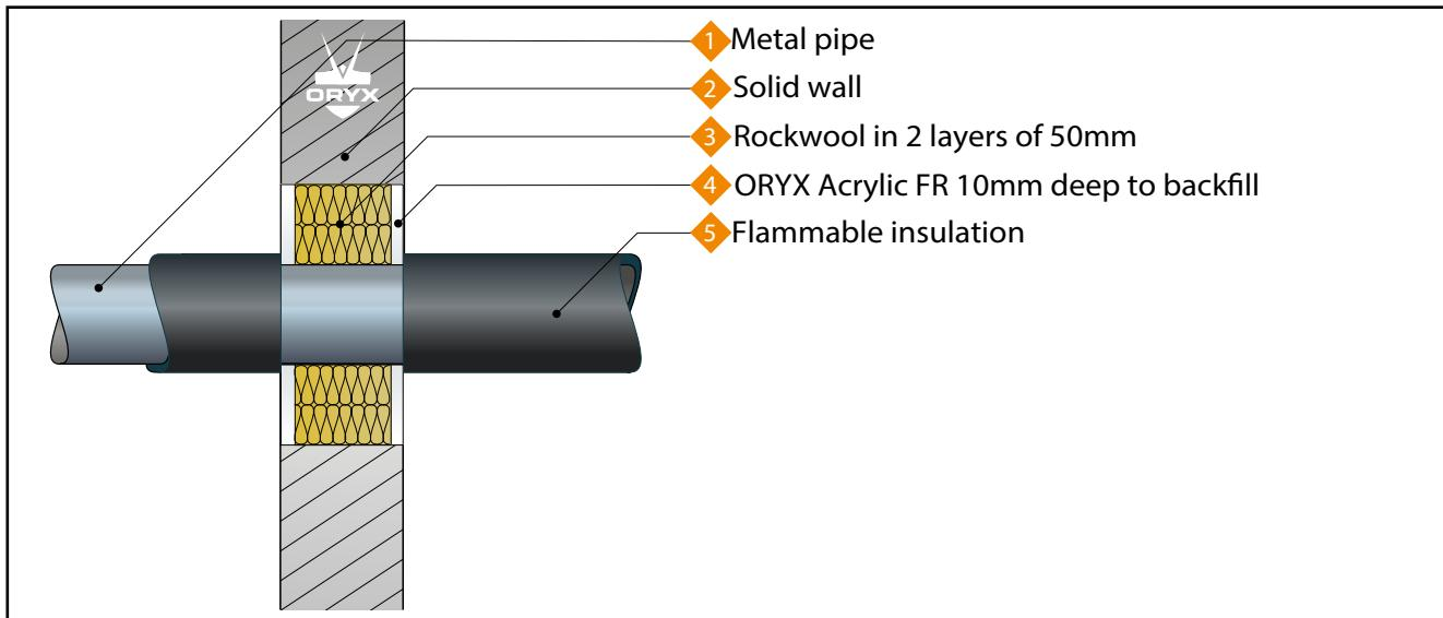
**A.1.1.1 Pipes with 'local interrupted' (LS) (min. 500 mm) or 'continuous interrupted' (CI) 19 mm thick Armacell Class O Armaflex insulation**
