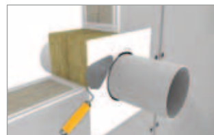
Smoothing of the surface with a spatula
