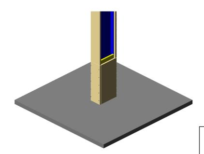
18 mm ORYX® Board strips, 100 mm wide, seam seals between vertical boards, stapled with divergent point staples 32 mm, centre-to-centre
