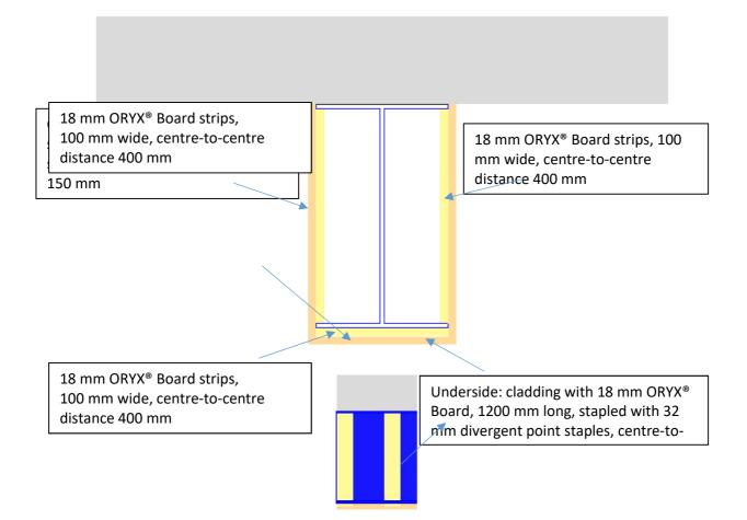
Underside: cladding with 18 mm ORYX® Board, 1200 mm long, stapled with 32 mm divergent point staples, centre-to-
