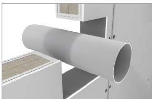
Reveals and rough opening must be cleaned
