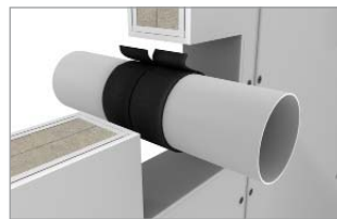
Wrapping* of both sides of the combustible pipe flush with the surface of the penetration seal
